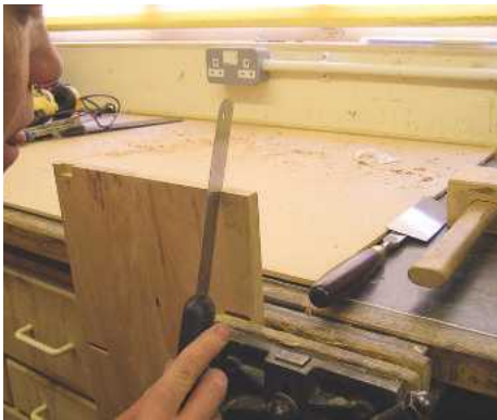
▲ Pic.4 ...in which the tails were formed using a small pull-saw...
